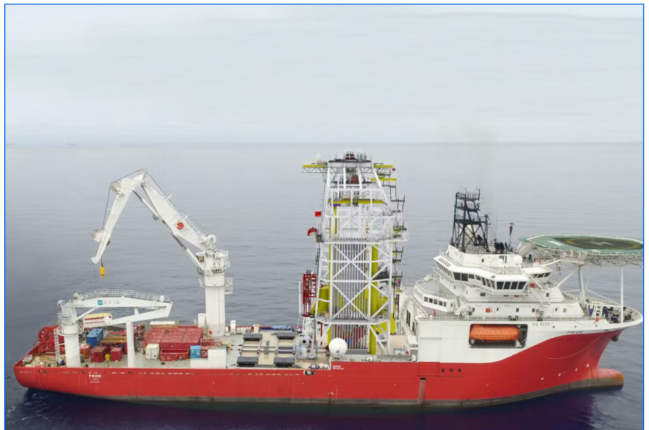
Image 1. An example of a Light Well Intervention Vessel (LWIV) used for P&A activities.
